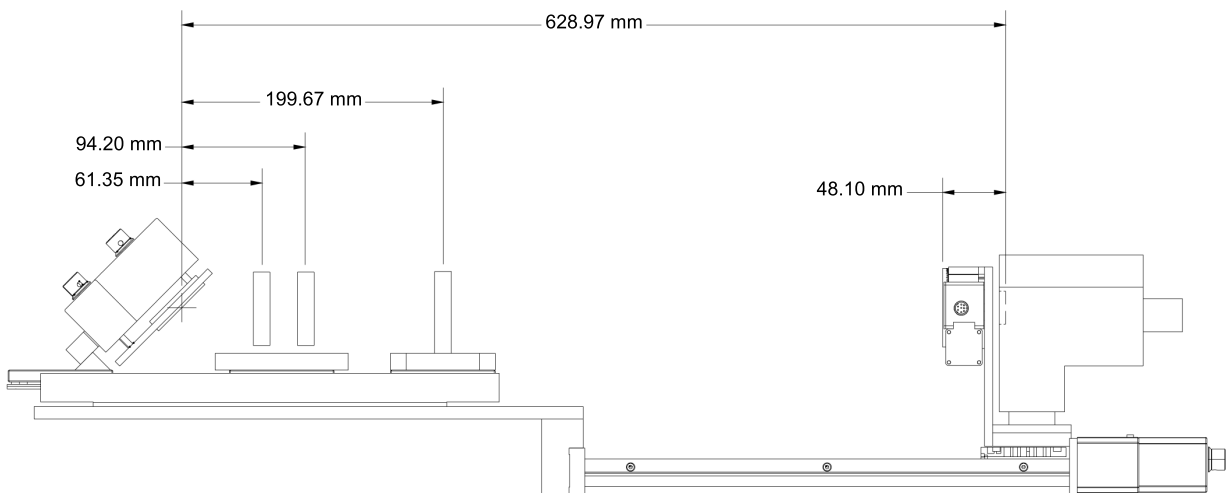
FIG. 5. A technical drawing of the optical system. From left to right is the folding mirror in the motorized holder, the lenses on flip stages for target imaging and angular distribution observation, the fixed bandpass filter, the Glan-laser polarizer in a rotation stage, and the camera mounted on a translation stage for the two observation positions.
