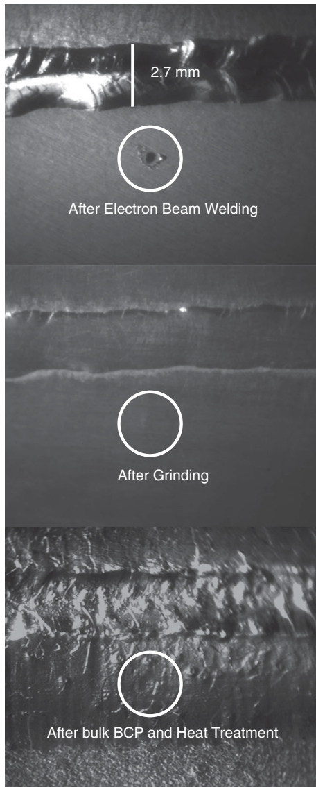
FIG. 2. Cure of a defect in cavity 3HZ004, appearing close to equator 9. Top picture shows the inspection after fabrication, middle picture after the local grinding and bottom picture after the bulk etching BCP process and heat treatment. The dimension of the weld seam is approximately 3 mm in width.
