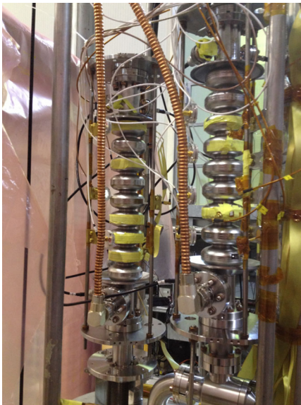
FIG. 9. Vertical insert with two cavities ready for vertical test, fully equipped with thermometers and second sound sensors.
