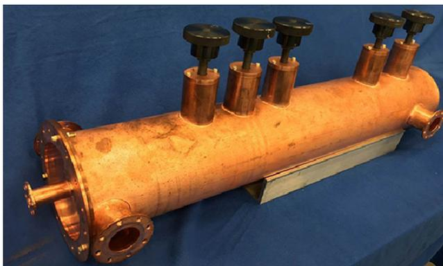
FIG. 13. Prototype cavity made of copper.
