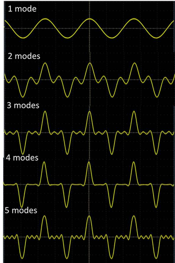
FIG. 22. The result of the odd harmonic modes combined one by one viewed on the oscilloscope display. Here the fifth mode is in the reverse phase to make the final kicking pulse more flat. The final working pulse is a flat-top kicking pulse which is the combination of a DC component and 10 continues harmonic modes separated in four cavities, here we just use five odd harmonic modes in the first cavity for a demonstration purpose.
