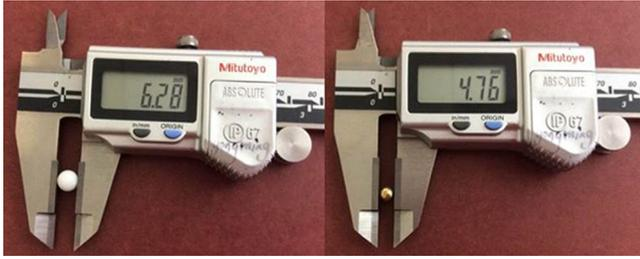
FIG. 18. Perturbing objects employed in the measurement with their dimensions measured by caliper. (Left: Teflon. Right: Brass).
