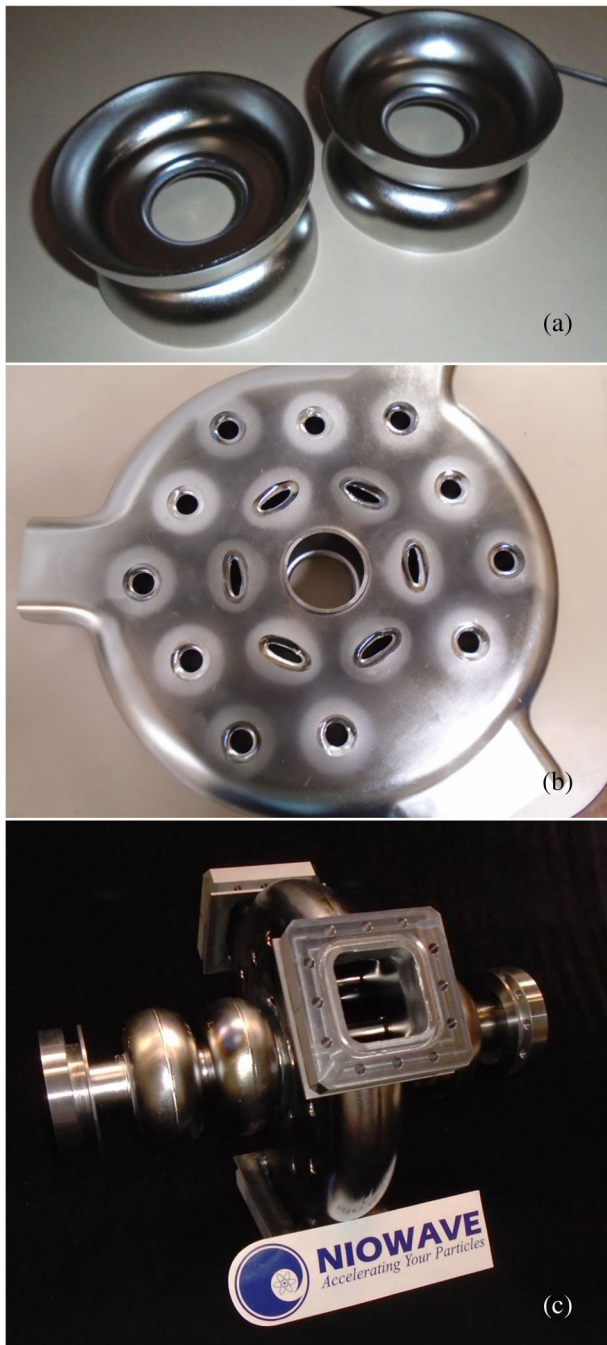
FIG. 8. Halves of the elliptical cells after being welded together at the irises (a). Photo of the PBG cell with welded rods (b). Final photo of the fabricated five-cell cavity (c).
