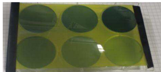
FIG. 5. EBT3 film irradiated with six different amounts of dose (0.5–4 Gy).
