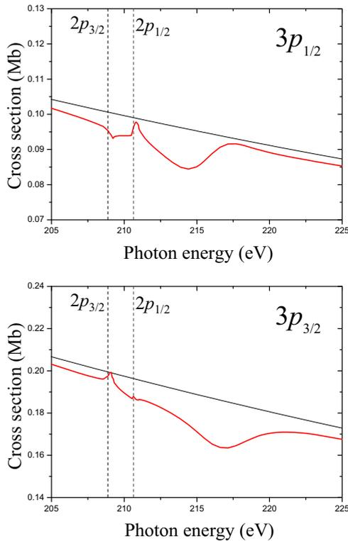
FIG. 1. Photodetachment cross sections for the  $3p_{1/2}$  subshell of  $\text{Cl}^-$  (upper panel) and the  $3p_{3/2}$  subshell (lower panel) in the vicinity of the  $2p$  thresholds calculated at the 14-channel (thick red curve) and 7-channel (thin black curve) levels as explained in the text. The  $2p$  thresholds are indicated by vertical dashed lines.
