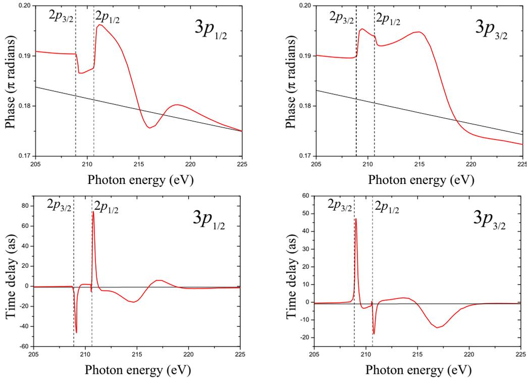
FIG. 3. Phases of the  $3p_{1/2}$  subshell of  $\text{Cl}^-$  (upper left panel) and the  $3p_{3/2}$  subshell (upper right panel) and time delays (lower left and lower right panels, respectively) in the vicinity of the  $2p$  thresholds calculated at the 14-channel (thick red curve) and 7-channel (thin black curve) levels as explained in the text. The  $2p$  thresholds are indicated by vertical dashed lines.
