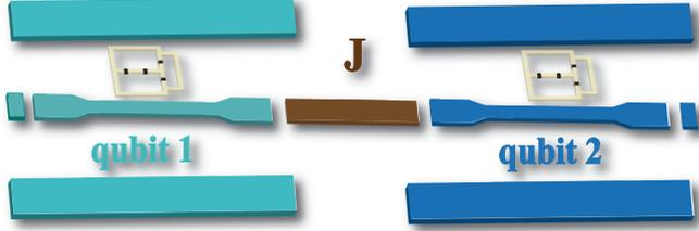
FIG. 1. Schematic of the experimental architecture. Two gap-tunable superconducting flux qubits are coupled to two neighboring interacting superconducting transmission line resonators, respectively.
