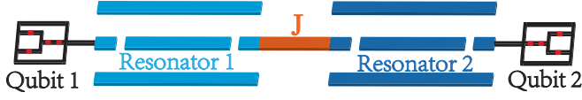
FIG. 1. Schematic of two directly coupled superconducting transmission line resonators, each coupled to a gap-tunable superconducting flux qubit. The flux qubit is made up of four Josephson junctions.
