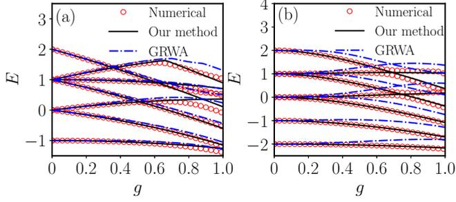
FIG. 1. The energy spectra of the system with (a)  $\Omega = 1.0$  and (b)  $\Omega = 2.0$ . The numerical result is obtained by an exact diagonalization of Hamiltonian Eq. (1). The results for our method and the GRWA are obtained by solving Hamiltonian Eq. (11) with an optimal  $\lambda = g/(\omega + \Omega)$  and  $\lambda = g/\omega$ , respectively.
