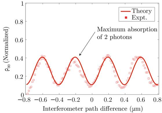
FIG. 3. Variation of the two-photon absorption coefficient ( $\rho_{00}$ ) as a function of the interferometer path difference, measured at the metamaterial sample. The squares represent the experimentally measured component, which has been interpreted using the theoretical model including losses. The solid line represents the theoretically calculated  $\rho_{00}$  component with no free parameters.
