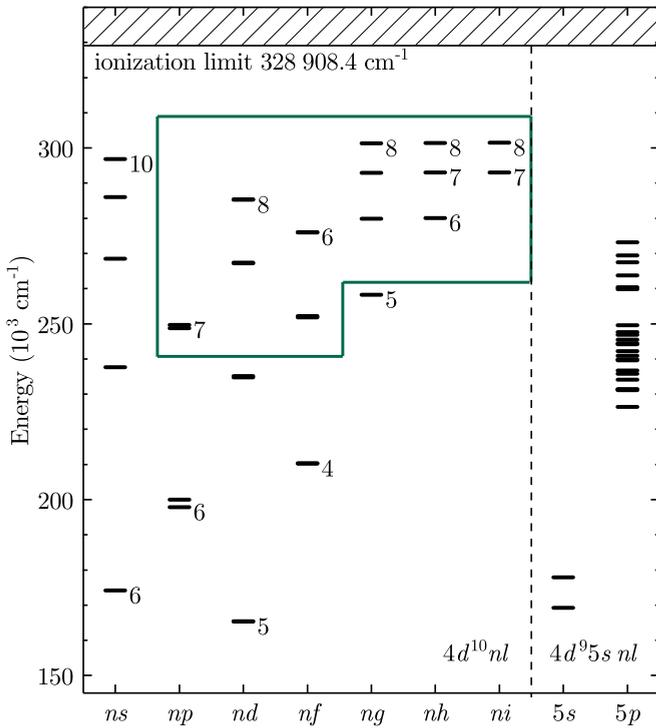
FIG. 6. Level diagram of Sn<sup>3+</sup>, drawn from 150 000 cm<sup>-1</sup> to the ionization limit at 328 908.4 cm<sup>-1</sup>. The ground state 5s, the 5p<sup>2</sup>P term, and multiply excited configurations lying near the ionization limit are omitted, as transitions to these levels occur outside the detection range of this study. The levels determined in this study are shown in the boxed area. Other levels are based on Refs. [24] and [30].
