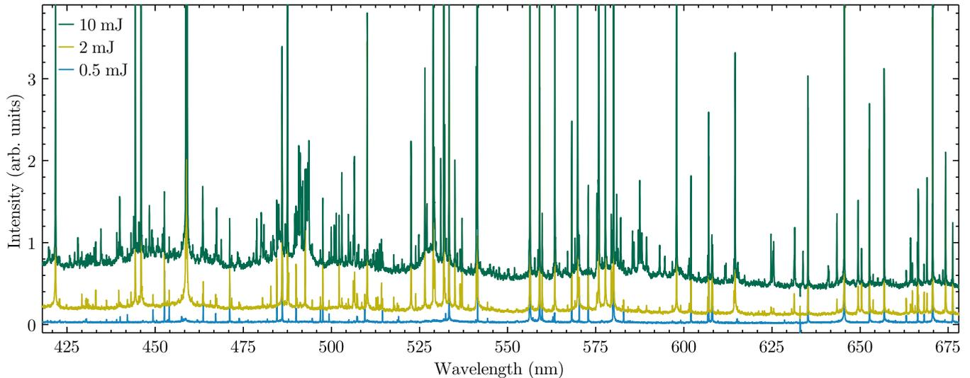
FIG. 2. Experimentally obtained Sn<sup>q+</sup> spectra for laser energies of 0.5 mJ (blue; lower), 2 mJ (yellow; middle), and 10 mJ (green; upper). The observable increase in the background level is due to increased continuum emission from the plasma at higher laser energies. Spectra shown are taken without spectral filters and, thus, include second-order contributions.
