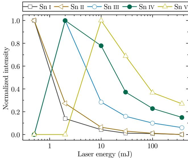
FIG. 4. Normalized scaled intensities of SnI–SnV lines as a function of the laser energy. The same lines as presented in Fig. 3 are used. Other SnI–SnV lines show a similar dependence on the laser energy.
