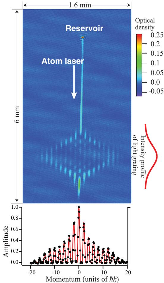
FIG. 2. The image in the top panel shows a typical time-of-flight absorption image of the atom-laser diffraction. The red curve drawn beside the image is the Gaussian intensity profile of the standing wave of light that forms the diffraction grating with which the atom laser interacts. The bottom panel shows the normalized population at different diffraction orders (up to  $\pm 18\hbar k$ ). Circles represent experimental data, whereas the solid line shows the numerical simulation.
