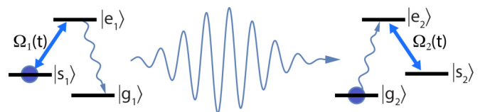
FIG. 3. Schematic depiction of a realistic scheme for the photon transfer between the two atoms. The first atom emits the photon, while the second atom fully absorbs it. By applying classical time-dependent control pulses \Omega_1(t) and \Omega_2(t) , the transfer can be initiated and the photon can be captured in the metastable state of the second atom, from which the photon can be read out using fluorescence techniques.
