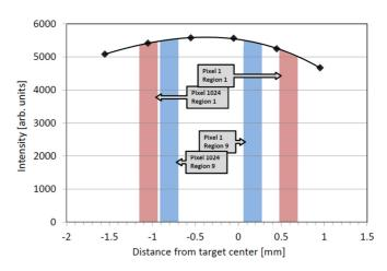
FIG. 1. C beam intensity profile employed to correct the  $K\alpha$  x-ray spectrum of Ca shown in Fig. 2. The red and blue vertical stripes represent the target areas seen by the pixels' columns 1 and 1024 for the CCD positions 1 (3650–3750 eV) and 9 (4350–4450 eV).
