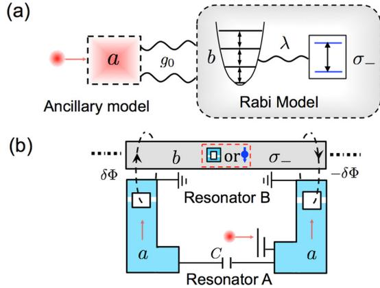
FIG. 1. (a) A hybrid quantum model including a Rabi model quadratically coupled to an ancillary cavity mode  $a$  with coupling strength  $g_0$ . (b) The implementation of this model in a superconducting circuit with the ability of simulating a quadratic optomechanical coupling [44] and coupling to a superconducting qubit or spin [49].
