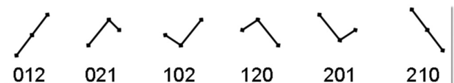
FIG. 7. The six possible ordinal patterns that can be obtained from D = 3 data points.
