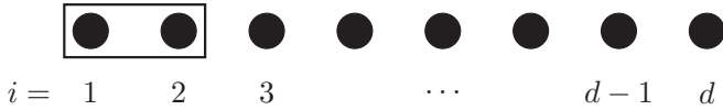
FIG. 1. Schematic representation of the block chain. Each dot represents one orbital (site). The rectangle represents a sub-block; in this case it contains two orbitals, and thus 4^2 = 16 possible configurations can be formed within the sub-block.
