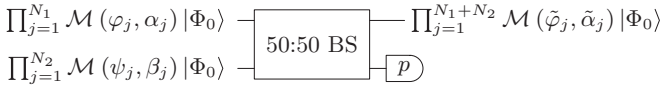
FIG. 3. Single round of a breeding protocol. The round takes approximate grid states defined by N_1 and N_2 measurement operators \mathcal{M} as inputs. It returns an approximate grid state with N_1 + N_2 (possibly changed) measurement operators. The second output port is subject to a homodyne measurement of the \hat{p} quadrature. The initial state |\Phi_0\rangle is chosen to be invariant under the action of a beam splitter, e.g., a squeezed vacuum state.
