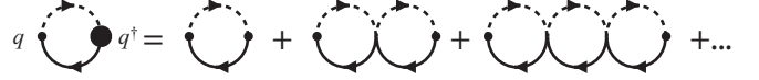
FIG. 6. The ring diagrams that are summed in the RPA calculation of G^{\text{RPA}} , Eq. (4.12). Note that the propagators are full mean-field propagators. The interaction joining two successive bubbles is the one in the second line of Eq. (4.11), namely, H_4 .
