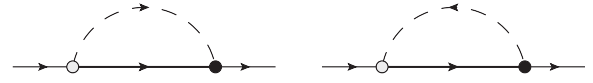
FIG. 1. Exact diagrammatic representation of self-energy \Sigma(P) in the weakly interacting Bose gas. The bold solid line represents the exact one-particle fermionic Green's function. The dashed line is the bosonic propagator in the Bogoliubov approximation. The dots stand for the zero-order (light) and the exact (black) vertices, respectively.
