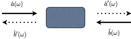
FIG. 1. Modes used to describe spectral filtering. There is one set of input modes of interest, which contains the light we are filtering, described by annihilation operators \hat{a}(\omega) . There is a second set of auxiliary input modes, which are assumed to be in the vacuum state, described by \hat{b}'(\omega) . There are two sets of output modes: The operators \hat{a}'(\omega) describe light transmitted through the filter, and that is the light we are going to perform measurements on with the aim to learn about the light in the input modes \hat{a}(\omega) . The other “reflected” modes, described by \hat{b}(\omega) , are available for further filtering operations (at different frequencies).
