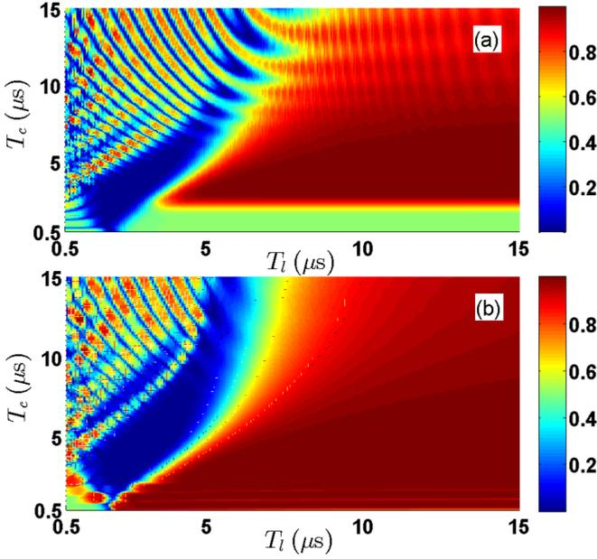
FIG. 4. The population  $P_f$  as a function of  $T_c$  and  $T_l$  in (a) the f-STIRAP process and (b) the f-STIRAP process with Lyapunov control. The pulse parameters are chosen as  $\Gamma/2\pi = 10$  MHz,  $\Omega_0 = 5\Gamma$ ,  $g_0 = 25\Gamma$ ,  $\nu = 30\Gamma$ ,  $d = 3/\Gamma$ . We take  $t = 16/\gamma$  for the simulation where the system has been a steady state.
