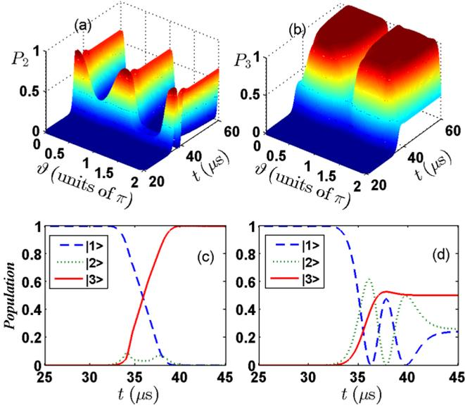
FIG. 2. The population (a)  $P_2$  and (b)  $P_3$  as a function of mixing angle  $\vartheta$  and evolution time  $t$ . The time evolution of population of bare state  $|k\rangle$  ( $k = 1, 2, 3$ ) in STIRAP, (c) with Lyapunov control at mixing angle  $\vartheta = 3\pi/2$  and (d) without Lyapunov control, where the parameters are  $T = 3.2 \mu\text{s}$ ,  $\tau = 0.7T$ ,  $\Omega_s^0 = \frac{5}{3}\Omega_p^0 = 1 \text{ MHz}$ .
