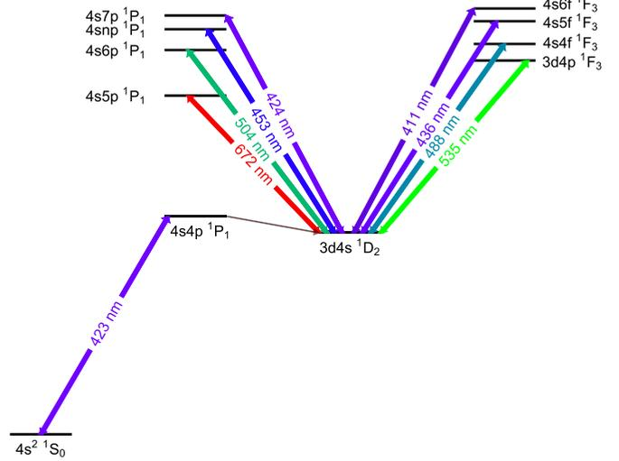
FIG. 3. Simplified calcium electronic level structure showing the eight repumping transitions considered here. All transitions except those at 504 and 535 nm have been studied experimentally. The overall best Ca MOT performance is found when pumping to a highly configuration-mixed state, labeled  $4snp\ ^1P_1$ , using the 453-nm  $4snp\ ^1P_1 \leftarrow 3d4s\ ^1D_2$  transition.
