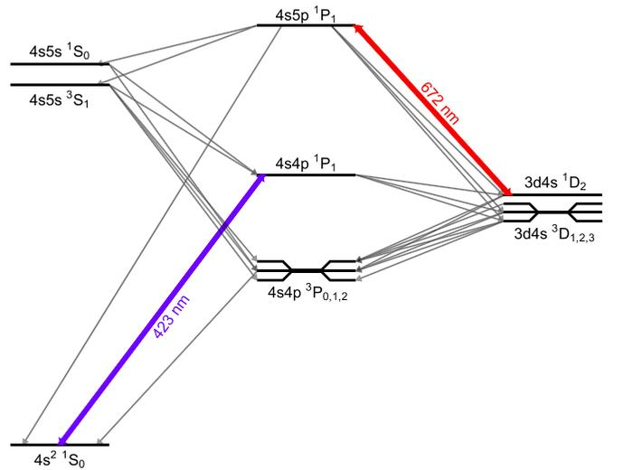
FIG. 2. Relevant level structure for operation of a standard calcium MOT. Laser cooling is accomplished on the 423-nm  $4s4p\ ^1P_1 \leftarrow 4s^2\ ^1S_0$  transition. Atoms that decay to the  $3d4s\ ^1D_2$  state are repumped back into the cooling cycle via the 672-nm  $4s5p\ ^1P_1 \leftarrow 3d4s\ ^1D_2$  transition, while those in the long-lived  $4s4p\ ^3P_{0,2}$  states are lost from the MOT.
