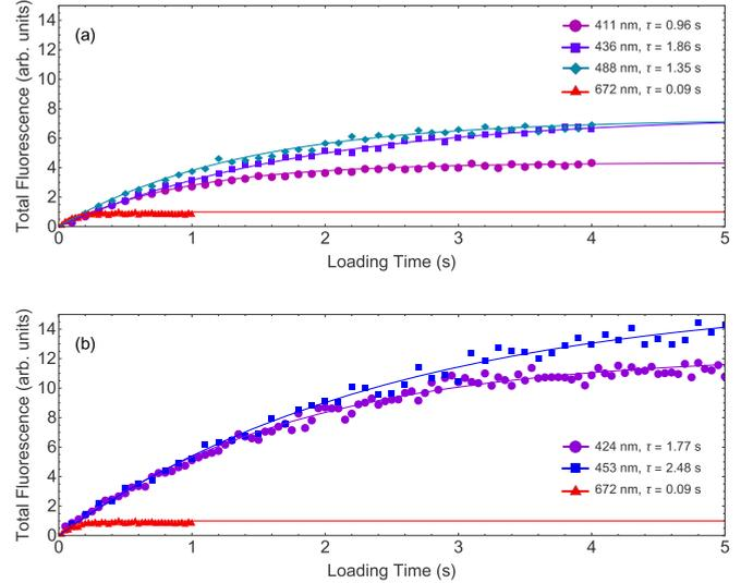
FIG. 5. Measured Ca MOT loading curves for (a) the  $^1F_3$  and (b) the  $^1P_1$  repump transitions, MOT fluorescence is plotted as a function of time elapsed after the cooling lasers are turned on; curves fitted to  $N(t) = R\tau(1 - e^{-t/\tau})$  are shown alongside the data.
