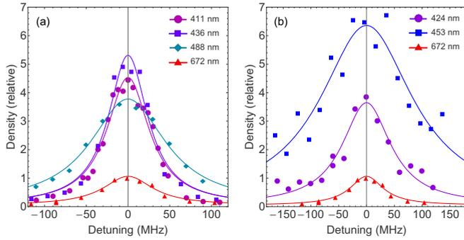
FIG. 4. Measured calcium MOT density as a function of the repumping laser detuning for (a) the  $^1F_3$  and (b) the  $^1P_1$  repump transitions. Experimental data are shown by symbols; Lorentzian fits, by lines. All measured densities are scaled to the peak MOT density achievable with the standard 672-nm repumping scheme.
