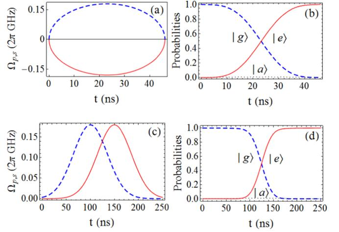
FIG. 4. (a) The designed Rabi couplings  $\Omega_p$  (blue dashed line) and  $\Omega_s$  (red solid line) vs time  $t \in [0, 46$  ns]. (b) The population transfer via the STA. (c) The Gaussian pulses in the STIRAP as functions of time,  $\Omega_p$  (blue dashed line) and  $\Omega_s$  (red solid line). (d) The Gaussian pulse-induced adiabatic population transfer from  $|g\rangle$  to  $|e\rangle$ .
