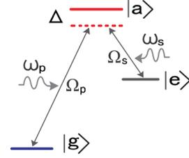
FIG. 3. In the case of two-photon resonance with a large detuning  $\Delta$ , a  $\Lambda$ -type interaction between the qutrit and the microwave drivings with frequency  $\omega_p$  and  $\omega_s$ , and the Rabi couplings are  $\Omega_p$  and  $\Omega_s$ , respectively.
