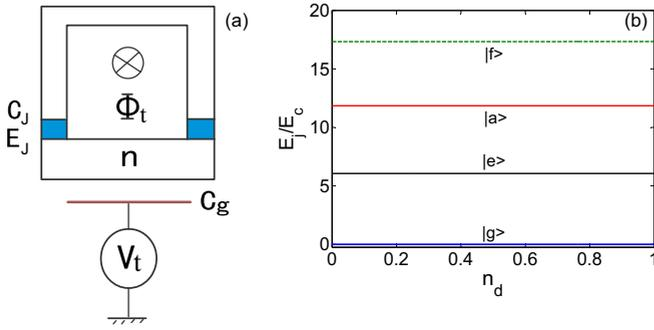
FIG. 1. (a) Schematic diagram of a transmon-regime quantum circuit. (b) The first four eigenlevels  $E_j$  (in units of  $E_c$ ) of the transmon system vs the static gate charge  $n_d$ , with  $j = g, e, a$ , and  $f$ . Here the system parameters are  $E_c/\hbar = 2\pi \times 1.05$  GHz and  $E_{Jd} = 20E_c$ . Level states  $|g\rangle$ ,  $|e\rangle$ ,  $|a\rangle$ , and  $|f\rangle$  are chosen at  $n_d = 0.5$ , and  $E_g$  has been taken as the zero-energy reference.
