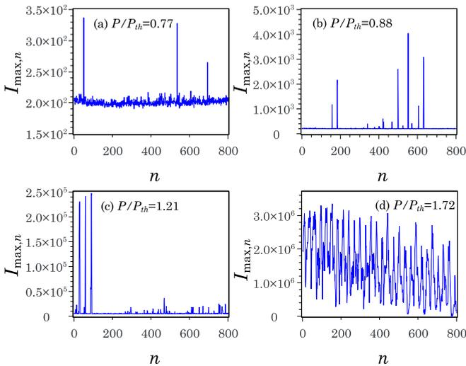
FIG. 3. Maximum intensity value  $I_{\max,n}$  (in arbitrary units) of the blocks  $n = 1, 2, \dots, M$  ( $M=800$ ) in which the  $N = 150\,000$  spectra displayed in Fig. 2 were divided. Data are shown for (a)  $P/P_{\text{th}} = 0.77$ , (b)  $P/P_{\text{th}} = 0.88$ , (c)  $P/P_{\text{th}} = 1.21$ , and (d)  $P/P_{\text{th}} = 1.72$ .
