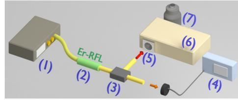
FIG. 1. Experimental setup of the Er-RFL system. (1) Fiber pigtailed semiconductor pump laser operating in the cw regime, (2) Er-RFL, (3) 1480 nm/1550 nm WDM, (4) power meter to measure the output power at 1480 nm, (5) RFL emission out to the spectrometer, (6) spectrometer, and (7) liquid-N<sub>2</sub> cooled InGaAs CCD camera.
