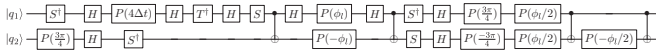
FIG. 1. Decomposition of one adiabatic step of the 2-qubit circuit into CNOT and single-qubit gates.
