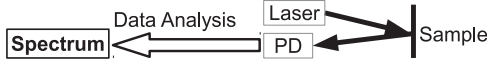
FIG. 1. Basic concept of the experiment: Laser light is shone on the sample mirror, and the reflected light is detected by a photodetector (PD). The output current of the photodetector is analyzed, and its power spectrum is computed.
