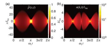
FIG. 1. Breathing-mode dynamics of the TG gas following a confinement quench. (a) Real-space density  $\tilde{\rho}(x,t) \equiv \rho(x,t)/\rho(0,0)$  and (b) momentum distribution  $n(k,t)/l_{\text{ho}}$  (where  $l_{\text{ho}} = \sqrt{\hbar/m\omega_0}$  is the harmonic-oscillator length) as functions of the dimensionless time  $\omega_1 t$ , for N=16 particles, quench strength  $\epsilon=35$ , and dimensionless initial temperature  $\theta_0 \equiv k_B T_0/N\hbar\omega_0 = 0.01$ .
