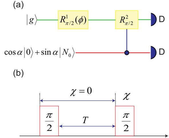
FIG. 2. (a) Schematic of the quantum delayed-choice experiment where the mechanical motion controls the second Ramsey rotation. (b) Sequence of microwave pulses and related procedures.
