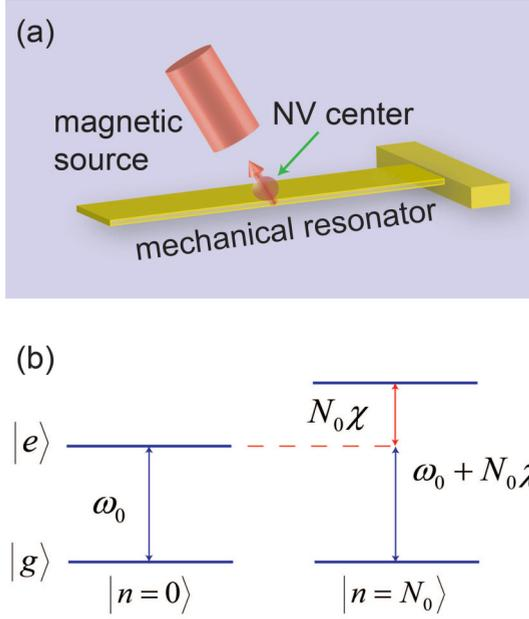
FIG. 1. (a) Schematic of a single NV center in a diamond resonator dispersively coupled to the mechanical motion. (b) Energy-level diagram of the spin-oscillator system. In the rotating frame of the resonator, the states  $|g, n\rangle, n = 0, 1, \dots$ , have the same energy.
