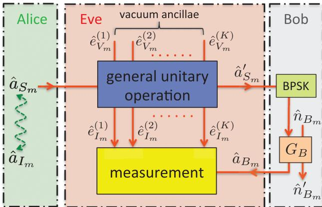
FIG. 5. Schematic of Eve's  $K$ -mode collective attack used to upper bound her Holevo information rate. BPSK: binary phase-shift keying.  $G_B$  amplifier gain. The dashed wavy line represents an entanglement that purifies the state of the  $\hat{a}_{S_m}$  mode.
