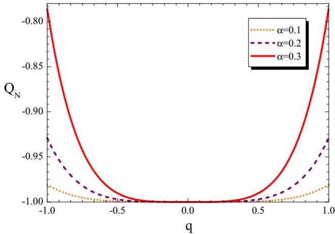
FIG. 5. Higher-order Mandel parameter of a NCHO as a function of  $q$  for different values of  $\alpha$ , with  $m = 1$  and  $N = 2$ .
