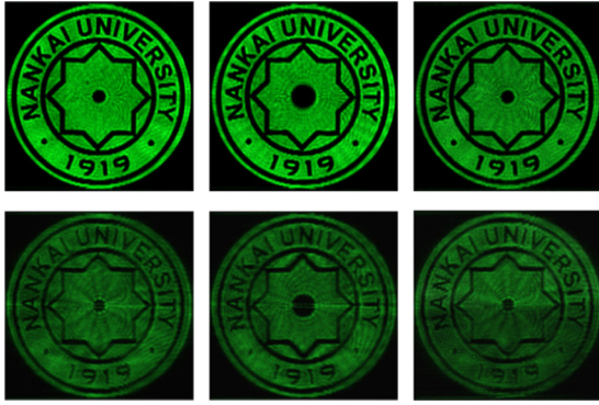
FIG. 6. The intensity patterns for three kinds of vector optical fields with the Nankai university logo obstructed by a sector-shaped filter with (b, \theta_0) = (\pi, \pi/2) in the spatial frequency plane. The first row shows three kinds of original vector fields, while the second row depicts the corresponding output fields. The first, second, and third columns correspond to the original vector fields with (m, T) = (10, 1) , (20, 1) , and (10, 0.3) , respectively.
