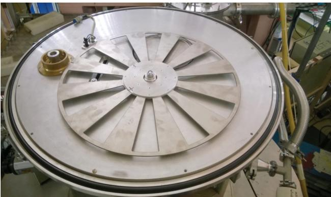
FIG. 4. Rotor of the Fourier modulator.
