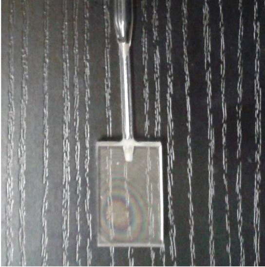
FIG. 1. The thin cell.
