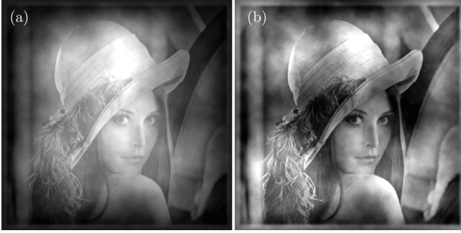
FIG. 5. Phase distribution in the image plane reconstructed using conventional TIE, Eq. (17), from two images with 1% noise (a); the same reconstructed distribution with the first 21 low-order Zernike components subtracted (b).
