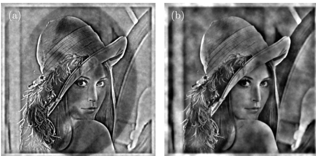
FIG. 6. Phase distribution in the image plane reconstructed according to Eq. (27) from two images with 1% noise, after two iterations (a), and after 20 iterations (b).
