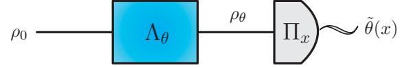
FIG. 1. (Color online) A general parameter estimation scheme in which a probe system prepared in an initial quantum state \rho_0 evolves under the quantum channel \Lambda_\theta to the output quantum state \rho_\theta . Note that \Lambda_\theta takes into account all decoherence processes that may be present in the setup. Following the evolution stage, the probe system is subjected to a general quantum measurement described by a POVM \{\Pi_x\} , which produces the measurement results x . These measurement results are then used to make an estimate of the parameter \theta via the estimator function \tilde{\theta}(x) .
