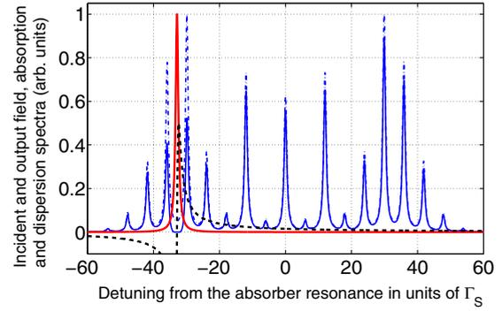
FIG. 3. (Color online) Spectra of the incident (dashed blue line) and output (solid blue line)  $\gamma$  radiation, resonant absorption (bold solid red line), and dispersion (bold dashed black line), corresponding to the time dependence of the intensity, shown in Fig. 2. All the spectra are plotted in the reference frame associated with the resonant absorber.
