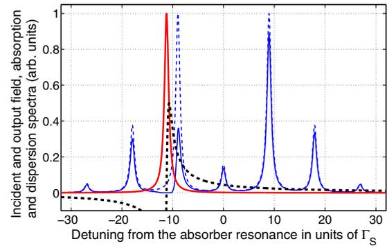
FIG. 7. (Color online) Spectra of the incident (dashed blue line) and output (solid blue line)  $\gamma$  radiation, resonant absorption (bold solid red line), and dispersion (bold dashed black line), corresponding to the time dependence of the intensity, shown in Fig. 6. All the spectra are plotted in the reference frame of the resonant absorber.
