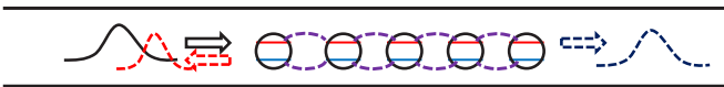
FIG. 1. (Color online) Single-photon transport through a linear atomic chain coupled to a one-dimensional photonic waveguide. The atoms can be coupled by the waveguide vacuum modes.
