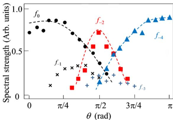
FIG. 4. (Color online) Strength of primary and sideband components in the  $-1-1$  line as a function of  $\theta$ . The dashed curves are guides for the eyes.  $f_0$  is a carrier component and  $f_n$  is the sideband component with the rotation frequency multiplied by integer  $n$ .
