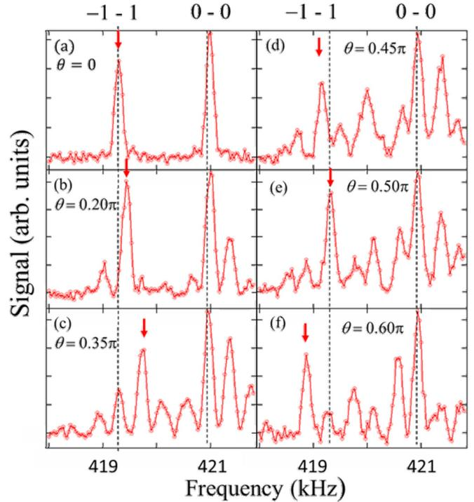
FIG. 3. (Color online) Spectrum from  $m' = -1$  to  $m = 1$  states (arrow) under the right-handed rotating magnetic field at 400 Hz with various angle  $\theta$  from the rotation axis, together with that from  $m' = 0$  to  $m = 0$  states as a reference. The frequency shifts zigzag as  $\theta$  increases. Dashed lines are their resonance frequencies at static magnetic field.
