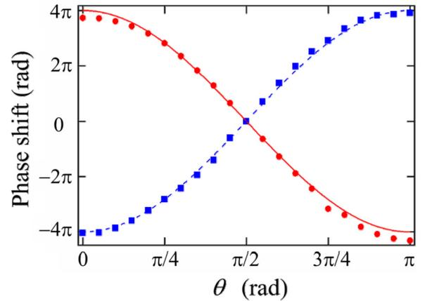
FIG. 2. (Color online) Observed Berry phase of spectrum from  $m' = -1$  to  $m = 1$  states for a whole rotation of the magnetic field using the atom interferometer as a function of angle  $\theta$  from the rotation axis. The phase shift is measured on the basis of the phase at  $\theta = \pi/2$ . (●) Right-handed rotation. (■) Left-handed rotation. Solid curve and dashed curve are  $4\pi \cos \theta$  and  $-4\pi \cos \theta$ , respectively.
