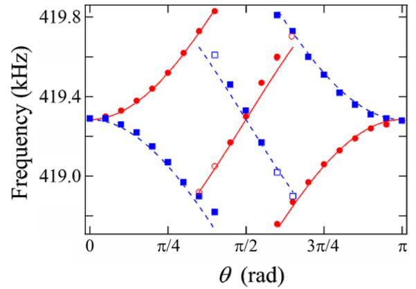
FIG. 5. (Color online) Observed frequency shift of spectrum from  $m' = -1$  to  $m = 1$  states as a function of angle  $\theta$  from the rotation axis, which is induced by the Berry phase evolving linearly in time. Rotation frequency of the magnetic field is 400 Hz. (●, ◐) Main and subpeaks for right-handed rotation. (■, □) Main and subpeaks for left-handed rotation. Solid lines and dashed lines are theoretical curves (see text).
