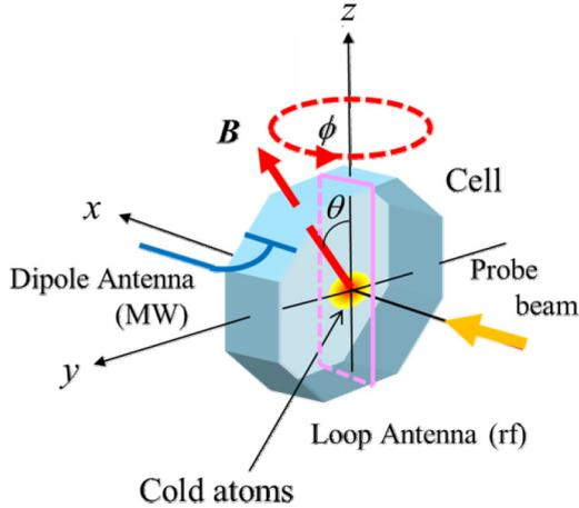
FIG. 1. (Color online) Experimental configuration. Cold atoms trapped in the cell are irradiated by the microwave (MW) and radio-frequency wave (rf) under the rotational magnetic field  $\mathbf{B}$  with an angle  $\theta$  from the  $z$  axis and a rotation angle  $\phi$ .
