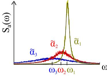
FIG. 2. (Color online) Simulated spectrum  $S_a(\omega)$  of the instantaneous model (15) with  $\text{Re } C = 10$ , noise autocorrelation coefficient  $R = 0.1$ , and three values of  $\tilde{\alpha}$ : 10 (blue), 5 (red), 1 (yellow) ( $C$ ,  $R$ ,  $S_a$ , and  $\omega$  are given in arbitrary frequency units). The noisy signal is the simulation result and the black curves are Lorentzian line shapes with widths  $\Gamma$  and center frequency shifts given by (29) and (31).
