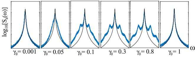
FIG. 3. (Color online) Simulated spectrum of the time-delayed model (33) with  $\text{Re } C = 10$  and  $R = 0.1$  (in arbitrary frequency units) at six values of  $\gamma_0$  (using a base 10 logarithmic scale for the y axis). The noisy signal is the simulation result and the black curves are Lorentzian line shapes with widths given by (29).
