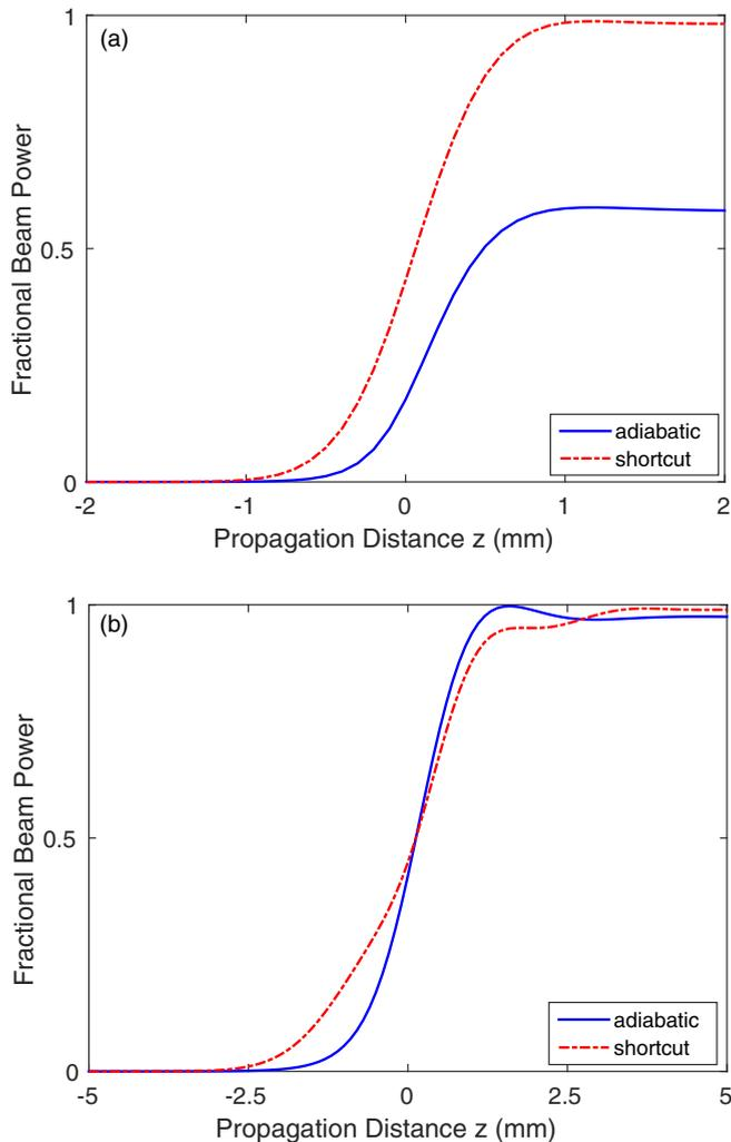
FIG. 4. (Color online) Fractional power output vs propagation distance for  $\Delta_0 = \kappa_0 = 1$  (a) for  $2L = 4$  mm and (b) for  $2L = 10$  mm.
