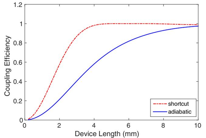
FIG. 5. (Color online) Coupling efficiency for adiabatic and STA coupler with varying device lengths. Parameters are the same as in Fig. 4.
