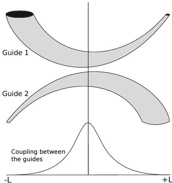
FIG. 1. Schematic for adiabatic directional coupler with Allen-Eberly scheme.  $\beta_1$  and  $\beta_2$  are propagation constants for waveguide one and two, respectively. Coupler length is  $2L$ . Maximum of the coupling occurs at  $L = 0$ .
