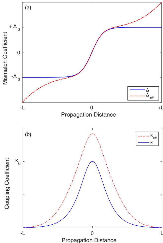
FIG. 2. (Color online) Spatial variation of (a) mismatch coefficient  $\Delta$  and  $\Delta_{\text{eff}}$ .  $\Delta$  varies from  $-\Delta_0$  to  $+\Delta_0$ , but  $\Delta_{\text{eff}}$  is greater towards the ends. (b) Coupling coefficients  $\kappa$  and  $\kappa_{\text{eff}}$ . Amplitude of  $\kappa_{\text{eff}}$  is greater than  $\kappa$ .
