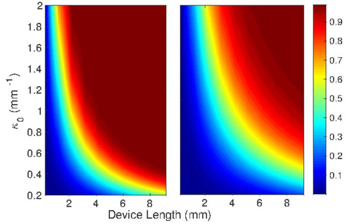
FIG. 3. (Color online) Contour plots for output power with varying  $\kappa_0$  and device length  $L$ . Shortcut (left) shows high fidelity over adiabatic coupler (right).
