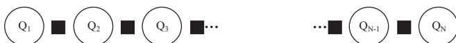
FIG. 5. The LNN arrangement of N qubits (represented as circles) with each qubit coupled only to its immediate neighbors (couplings represented as squares). The couplings may or may not be switchable. Qubits are labeled Q_1, Q_2, \dots, Q_N .
