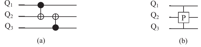
FIG. 1. (a) Two successive CNOT gate operations, which perform the C^2(\mathbf{P}) gate operation as given by Eq. (1). For both gates, qubit Q_2 is the target qubit. (b) Our representation of the C^2(\mathbf{P}) gate as a single elementary gate operation. Here the vertical line connecting qubits Q_1 , Q_2 , and Q_3 shows that the gate operation involves all three qubits. To distinguish between the two controls and the target, a square with the letter P is placed on the target qubit. This indicates that after the gate operation, the state of the target qubit Q_2 will hold the parity of the three qubits, while the states of the two-control qubits Q_1 and Q_3 remain unchanged [Eq. (1)].
