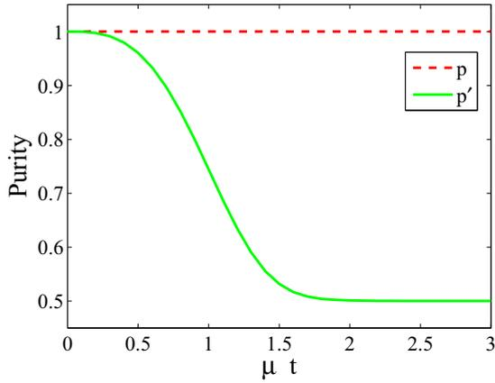
FIG. 3. (Color online) The purity versus the dimensionless parameter  $\mu t$ . The results were obtained by calculating the master equation with the coherence control field  $\Omega(t)$  (red solid lines) and without the coherence control field (green dashed lines). The figure is evaluated for  $\mu = \gamma$  and  $\nu = 2\pi\gamma/3$ .
