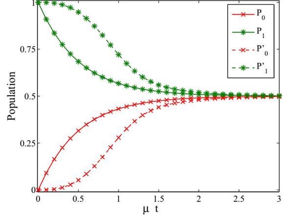
FIG. 2. (Color online) The population of the ground state  $|0\rangle$  (red cross lines) and the excited state  $|1\rangle$  (green star lines) versus the dimensionless parameter  $\mu t$ . The results were obtained by calculating the master equation with the coherence control field  $\Omega(t)$  (solid lines) and without the coherence control field (dashed lines). The figure is evaluated for  $\mu = \gamma$  and  $\nu = 2\pi\gamma/3$ .
