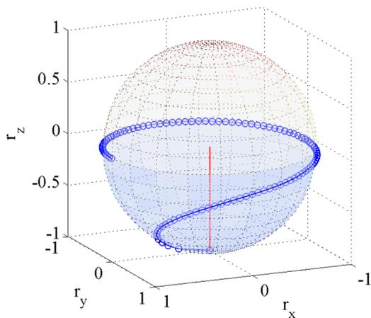
FIG. 4. (Color online) The evolution of the quantum state on the Bloch sphere. The results were obtained by calculating the master equation with the coherence control field  $\Omega(t)$  (blue curved line) and without the coherence control field (red straight line). The figure is evaluated for  $\mu = \gamma$  and  $\nu = 2\pi\gamma/3$ .
