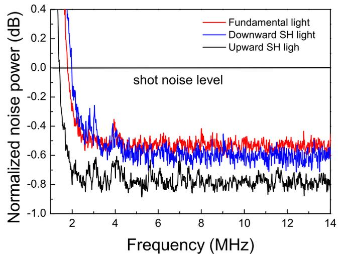
FIG. 2. (Color online) Normalized noise spectra of fundamental light, upward SH light, and downward SH light. The resolution bandwidth and the video bandwidth of the spectrum analyzer are 300 kHz and 300 Hz, respectively. All results are obtained with 5 times averaging.
