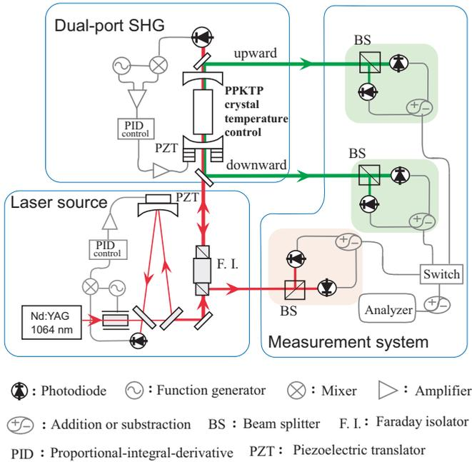
FIG. 1. (Color online) Schematic diagram for generation of tripartite-quantum-correlated amplitude-squeezed beams.
