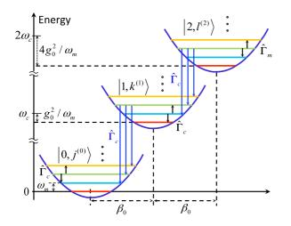
FIG. 1. (Color online) Schematic energy diagram and systembath coupling of the optomechanical system (with only the zero-, one-, and two-photon subspaces shown). The arrows indicate transitions induced by cavity (blue) and mechanical (black) bath modes.
