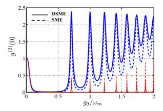
FIG. 3. (Color online) Photon correlation  $g^{(2)}(0)$  vs  $g_0/\omega_m$  at detuning  $\Delta_0 \equiv g_0^2/\omega_m$  and driving amplitude  $E_0 = 0.1\kappa$ . Thin (red) curves are for  $n_{\rm th} = 0$ ; thick (blue) curves are for  $n_{\rm th} = 10$ . Other parameters are  $\kappa = 0.005 \omega_m$  and  $\gamma_m = 0.0033 \omega_m$ .
