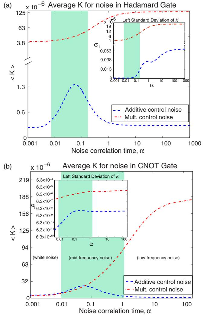
FIG. 2. (Color online) Averages and left standard deviations (inset) of robustness distributions of the optimal Hadamard gate (a) and CNOT gate (b). The shaded regions denote midfrequency noise, where noise power is centered around the same spectral domain as system dynamics ( $\omega \in [6, 50]$ ). White noise and low-frequency noise lie to the left and right of this region, respectively.
