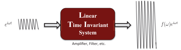
FIG. 2. (Color online) Any linear time-invariant process transforms an input signal of frequency \omega to an output signal of the same frequency. In other words, linearity together with time invariance implies that the process cannot change the frequency of the input. It follows that any linear time-invariant system can be uniquely specified by a complex function f(\omega) specifying the change in amplitude and phase of the mode \omega . This explains why Fourier analysis is extremely useful for the study of these processes.
