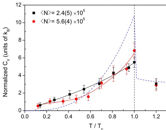
FIG. 4. (Color online) The normalized heat capacity versus the average number of atoms  $\langle N \rangle$  as a function of reduced temperature ( $T/T_c$ ) for two different  $\langle N \rangle$ . Solid lines are interpolations of the data. The blue dashed line is the theoretical curve for the finite- $N$  corrected, large  $N$  case.
