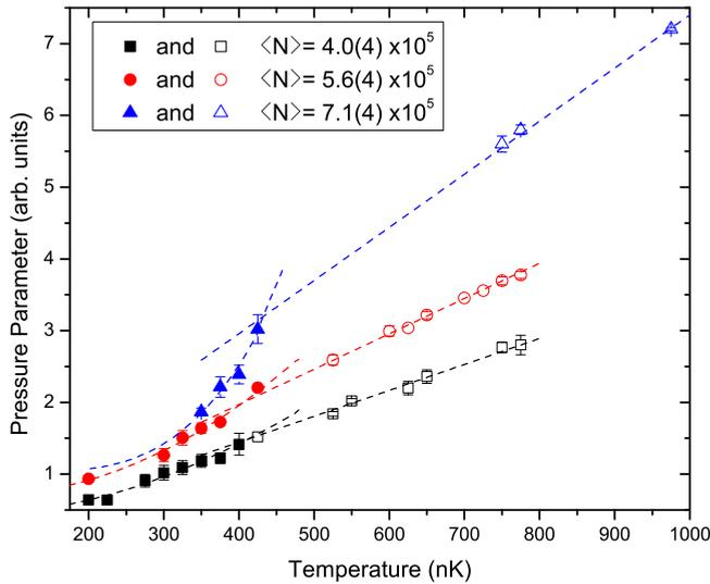
FIG. 1. (Color online) *Pressure parameter* as a function of temperature for three different averaged particle number  $\langle N \rangle$ . For each  $\langle N \rangle$ , the crossing between a linear fitting for thermal points (open symbols) and the interpolation or extrapolation of points with measurable condensate fraction (solid symbols) determines the critical point.
