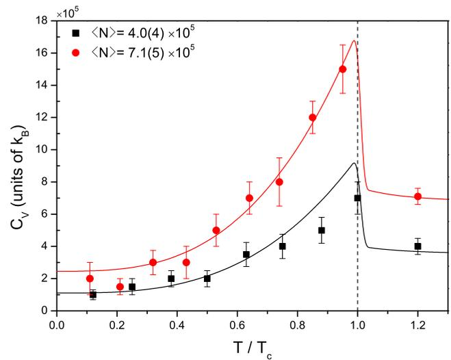
FIG. 2. (Color online) The heat capacity versus the reduced temperature is plotted around the condensation temperature  $T_c$  for two different atom numbers. The experimental points are extracted from diagram of Fig. 1, via Eq. (4). The lines result from Eqs. (10) and (14) [8], where  $N$  is the only adjustable parameter.
