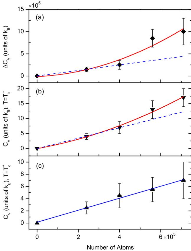
FIG. 3. (Color online) Dependence of the heat capacity around the critical temperature on the total number of atoms: (a) the  $\Delta C_V$  jump, (b)  $C_V(T_c^-)$ , and (c)  $C_V(T_c^+)$ . Dashed line is the theoretical result for a weakly interacting, large  $N$ , case and solid lines are only eye guides.
