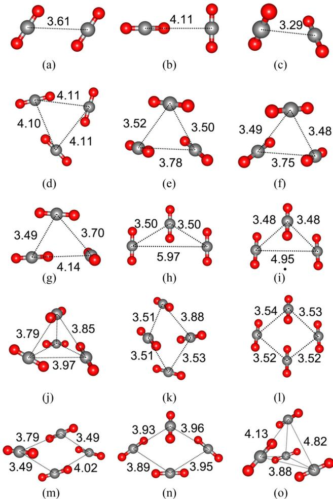
FIG. 1. (Color online) Predicted low-energy structures of CO<sub>2</sub> dimers, trimers, and tetramers.
