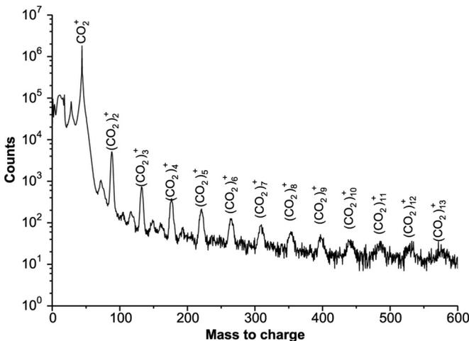
FIG. 2. Time-of-flight mass spectra of a supersonic carbon-dioxide beam irradiated by 780 nm, 25 fs laser pulses at an intensity of  $5 \times 10^{14}$  W/cm<sup>2</sup>.
