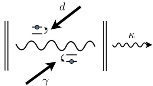
FIG. 1. (Color online) A pictorial representation of the model. Emitters lose energy at a rate  $\gamma$  while energy is pumped in at a rate  $d$ . Photons can leave the cavity after a time  $\kappa^{-1}$ .
